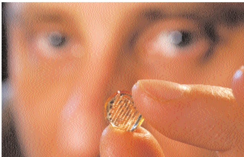
Mark Prausnitz, a professor in Georgia Tech's School of Chemical and Biomolecular Engineering, holds an array of polymer micro-needles that are approximately 1000  $\mu\text{m}$  tall.
