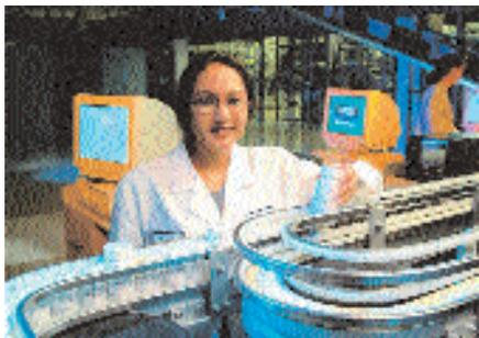
At Merck-Medco's automated pharmacy in Willingboro, New Jersey, bottle movement, filling, capping, and labeling are governed by a central computer system and bar coded components.
