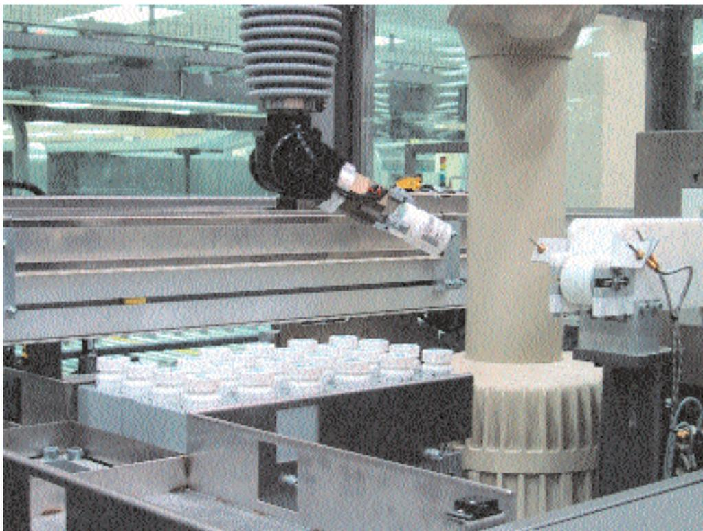
After filling and capping, a robot arm plucks each prescription bottle from its carrier and sets it on a conveyor for the trip to the consolidation point, where it is swept into a mailing bag along with personalized patient instructions and billing information.
