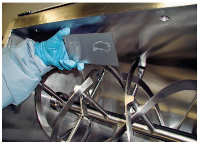
**Figure 2:** Equipment inspection using spotted plates.
