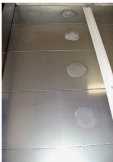
**Figure 1:** Representative residues on stainless steel.
