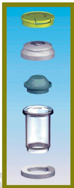
**Figure 1:** The five vial elements are (from bottom to top): the bottom ring for mechanical stability and processing; the vial body containing the liquid; the stopper that can be resealed with a laser; the top ring, which ensures closure integrity between the vial body and stopper; and the flip-top cap to protect the piercing area.
