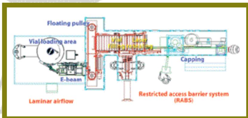
**Figure 4:** An overview of a production line for closed vials. First, under soft-wall laminar airflow, boxes of vials are opened mechanically on the loading table, and the vials' top surface is sterilized by an electron beam. Then, in the RABS, the vials' linear movement is converted to a parallel movement by a floating pulley. The vial filling and the laser resealing are performed on the transport bars, and then the vials are capped.
