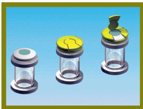
**Figure 3:** The sterile, ready-to-fill vial is delivered uncapped (left). After filling, the vial is capped (middle) inside an isolator. To use the vial, the central part of the flip-top cap is removed (right), exposing the large puncture area that has been kept sterile by the circular rib.
